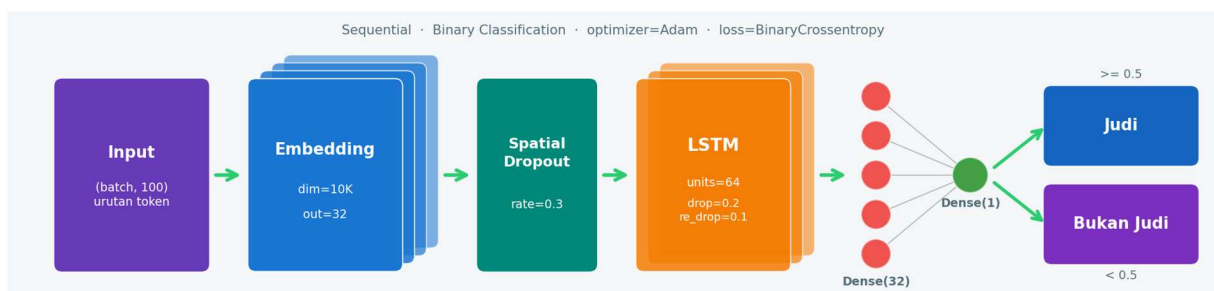
Figure 1. LSTM Architecture used for classifying OCR-extracted text.
